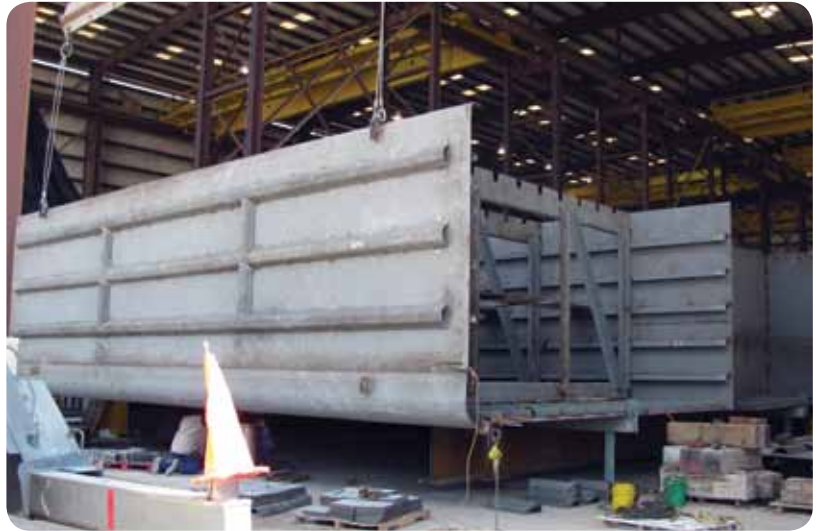
The new 250ft x 72ft x 12ft deck barge currently under construction at Conrad Industries.
