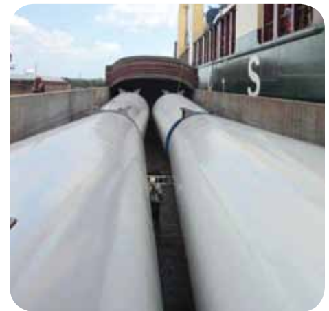
Windmill tower sections loaded to barge.
